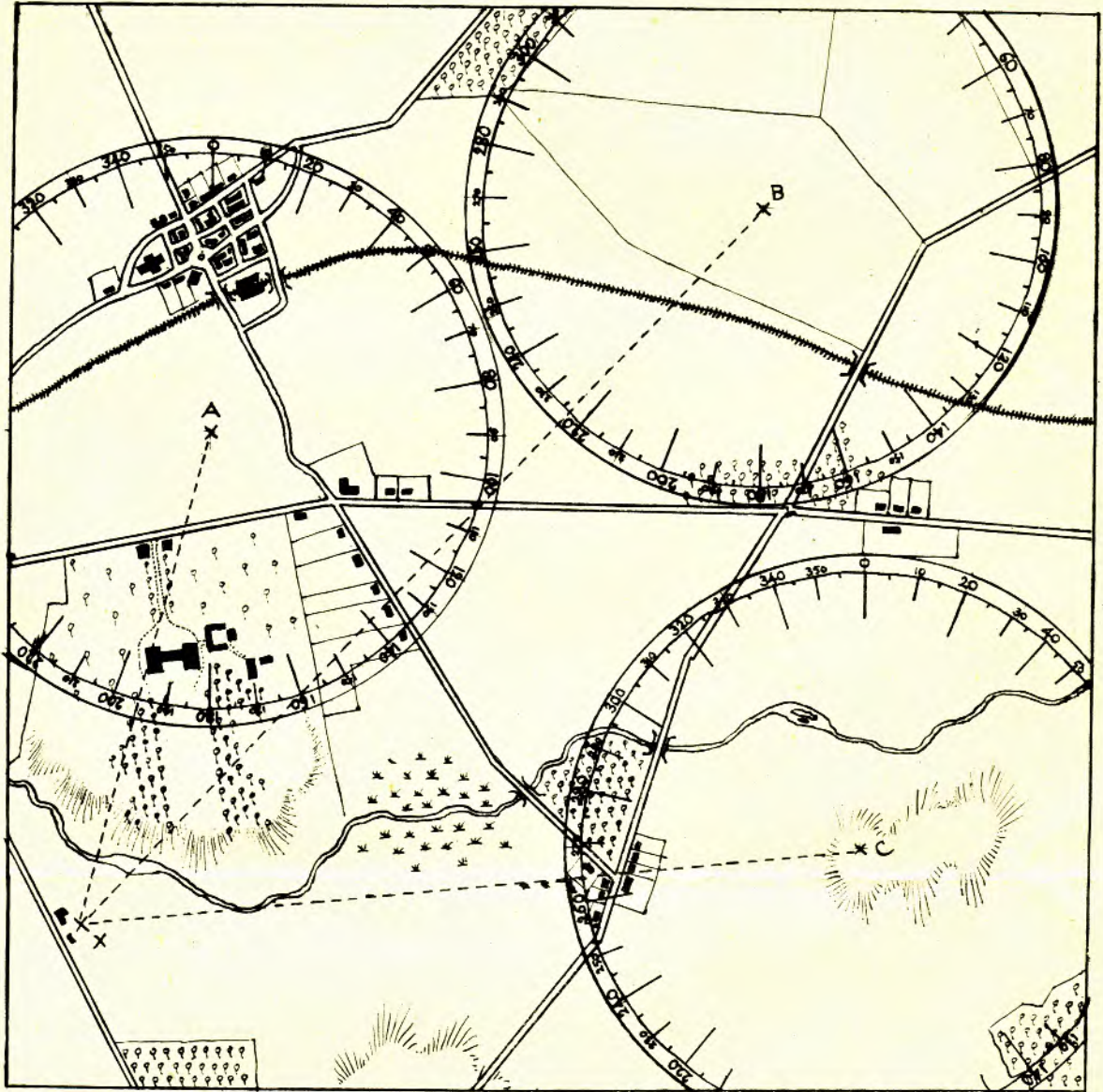
DIAGRAM OF MAP AT KEY POST ILLUSTRATING BEARINGS TAKEN FROM POSTS A, B, & C OF INCIDENT AT X.
